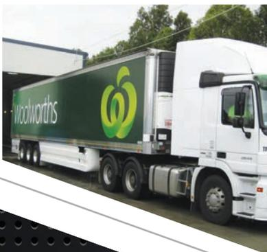
1. FuelSkirts are developed in multi-sized panels for easy installation under a truck body or trailer and limits the impact on the flat surface. FuelSkirts improve truck performance, stability and fuel consumption.
