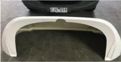
1. FUELSCOOP fitted to European LCV Cab-chassis have a fully bonded moulded base mounting system. Not only does this avoid damaging the cab, it also means the load is spread over total cab width and depth.
