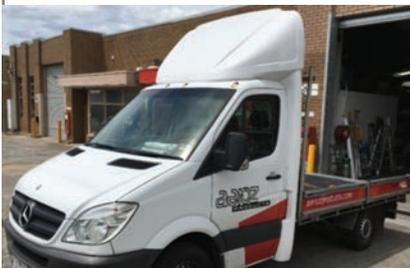
4. FUELSCOOP for European LCV Cab-chassis can be enhanced by means of upgrading to a FUELSCOOP Full Aero Kit. The FUELSCOOP Full Aero Kit combines the fully moulded roof device with left and right cab-extendors that are angled to suit the base of the FUELSCOOP. Not only do these look great they assist deflection of the airflow out and away from the front of the truck body.
