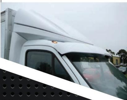
5. To compliment the performance of FUELSCOOP, AeroTrans Australia developed a fully moulded 'flow-through' Sunvisor, that is not only practical to shield from bright light, but also acts like a blade to assist laminar flow.
