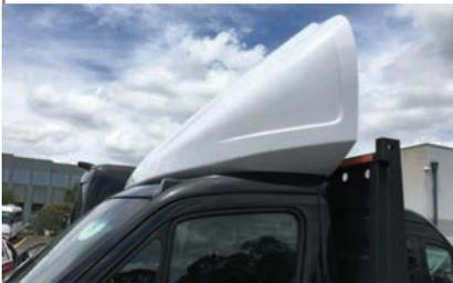
2. FUELSCOOP fitted to European LCV Cab-chassis has been designed for superior airflow from cab windscreen minimising likelihood of turbulence in transition. The consistent flow from cab to FUELSCOOP and beyond assists over-deflection in case of higher truck bodies.
