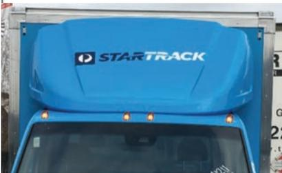
3. FUELSCOOP is designed with a 'cut' as can be easily seen in frontal photos. This design redirects airflow outwards causing a 'streaming' effect. This intensified airflow streams along the FUELSCOOP, minimising turbulence and providing a laminar flow, improving truck safety by substantially assisting vehicle stability.
