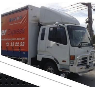
1. FUELSCOOP fits to Mitsubishi-FUSO cabs by a moulded base mounting system. It picks up Mitsubishi factory installed mount points, ensuring a no-risk installation.
