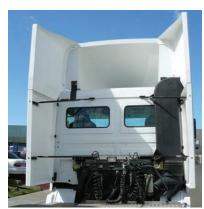
2. Fuelscoop Full Aero-Kits, in addition to their overall visual and performance appeal, are without excessive weight. The total weight of under sixty kilograms is achieved by means of design. This proven design means that the need for heavy steel brackets is eliminated. The load is spread over the total mounting surface and is trouble free.
