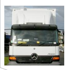
3. A frontal view of Fuelscoop exposes a 'cut' that redirects the airflow outwards causing a 'streaming' affect. With the Full Aero-Kit this intensified airflow stream passes over the extenders to a final 'kick' at their rear edge, assisting the flow onto the truck body, improving the truck's safety, increasing performance and reducing fuel consumption.
