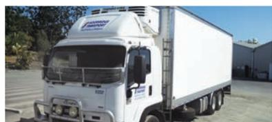
1. FRIDGESCOOP fits to truck cabs by a moulded base mounting system, or covered bracket system for smaller cabs. It picks up on factory installed mount points.
