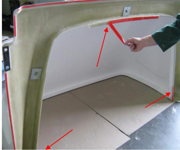
6. Slightly peel the edges of remaining double sided tape strips and tape them to the outside the part.
