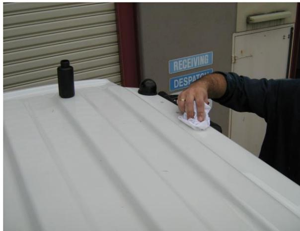
Clean these areas using Tite-R-Bond 2287A (supplied) using a clean lint-free rag. Ensure the bonding area is completely free of dust.
