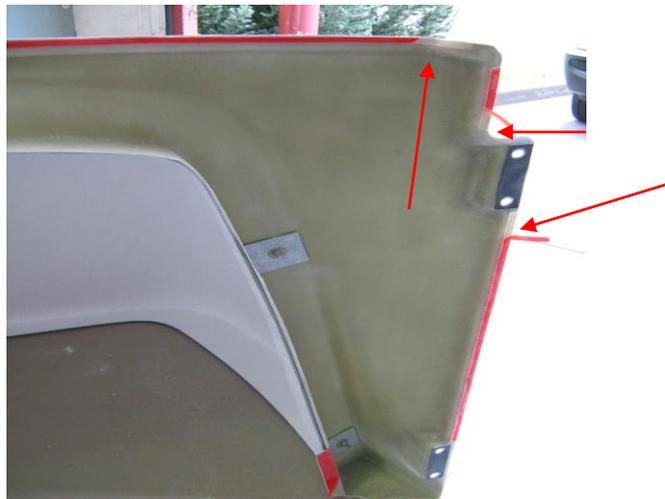
7. Place some spacer blocks on the cab roof between each tapped hole. Place the Fuelscoop on the cab roof ensuring the kit does not contact the roof. Screw in the 8x40mm set screws supplied. You may need to enlarge the holes if the bolts don't screw in easily.
